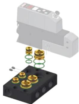
The multiple manifolds fit all sizes of MFE ejectors. It allows to mount 2-5 ejectors easily, quickly and compactly. To prepare for a potential increase in the number of ejectors on the multiple manifolds, a blind plate is available to reserve one position for this purpose. The manifold can be connected to the air supply (G3/8") on either side.
